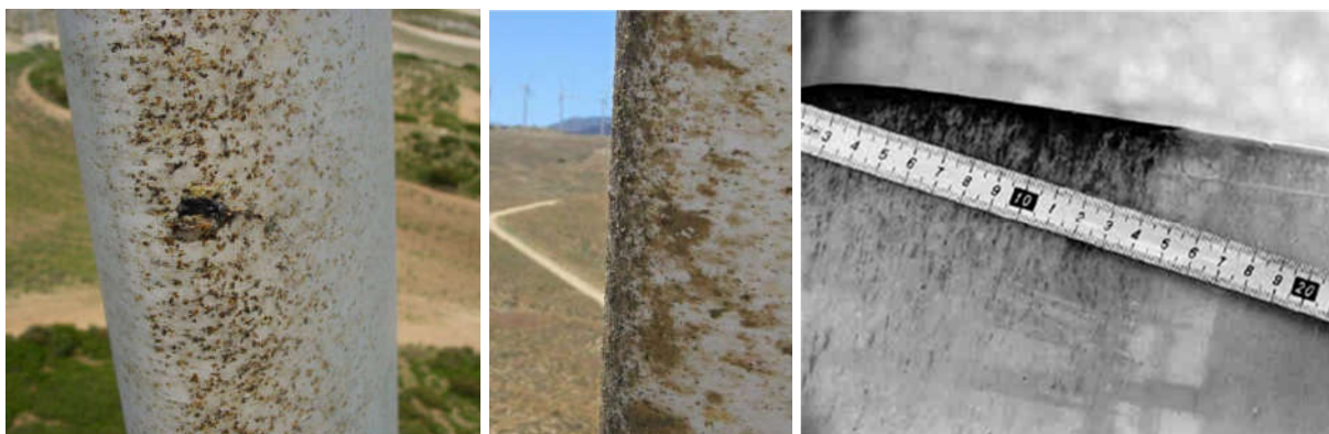
Figure 3: Examples of insect residues found on wind rotor blades. Left: Deposits of a swarm of the beetle Omophlus lepturoides (BladeCleaning 2018). Center: Unidentified insect roughness on rotor blades (Wilcox et al. 2017). Right: Soiled leading edge of a rotor blade near to the blade tip (Hinsch & Westermann 1996).
